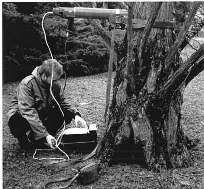
Figure 5. Frank Rinn using the first kind of mobile resistance drills (“DENSITOMAT”) for tree-ring analysis of a Metasequoia glyptostroboides in Heidelberg Botanical Garden (1987). Providing constant supply voltage, the power consumption of the drill was electrically measured, recorded and plotted on paper in 1:1 scale.
