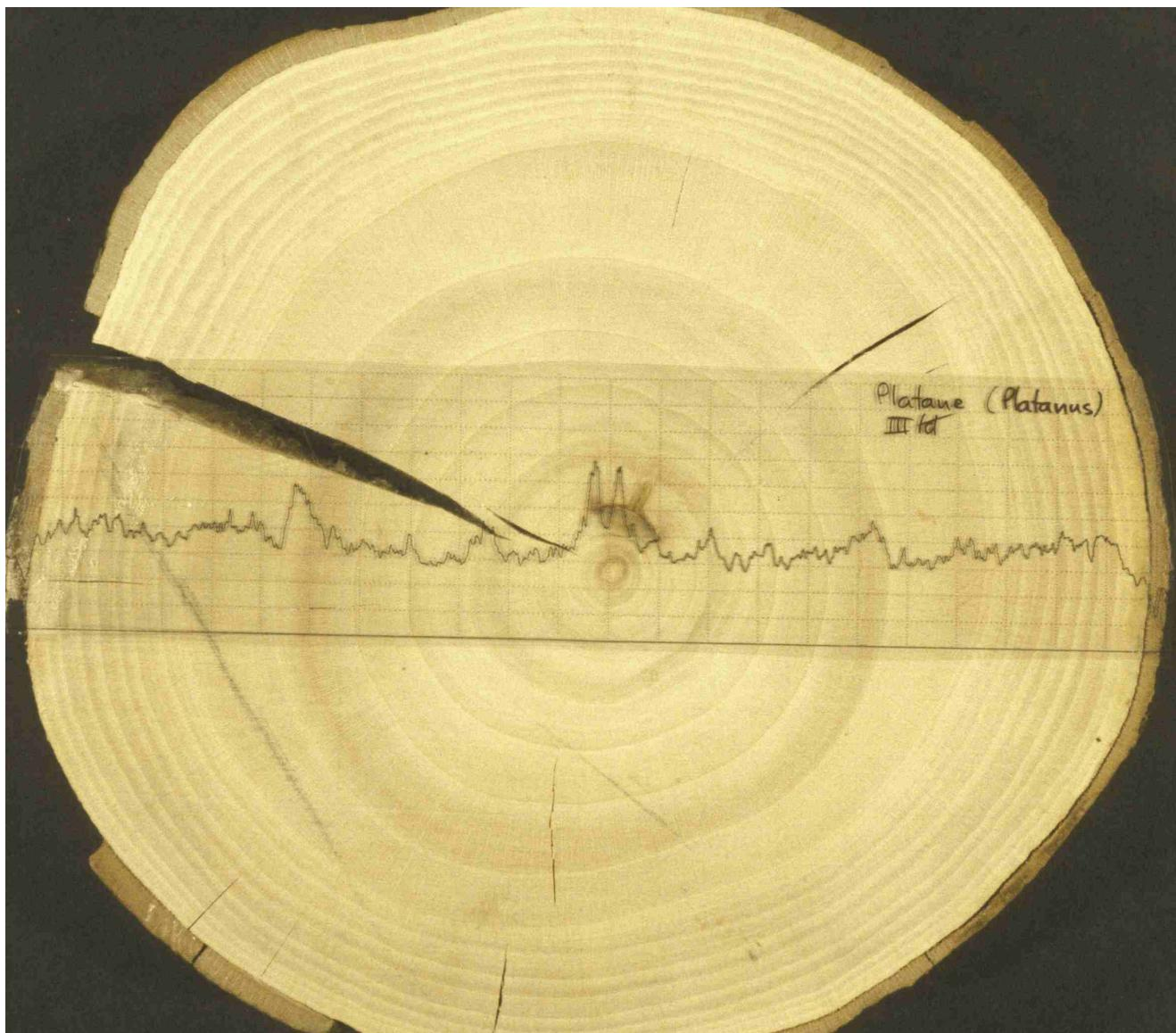
While conifers are mostly much softer in the center, ring-porous trees are much stronger in the center and diffuse porous trees are more homogenous in their density and strength distribution in a cross-section.
