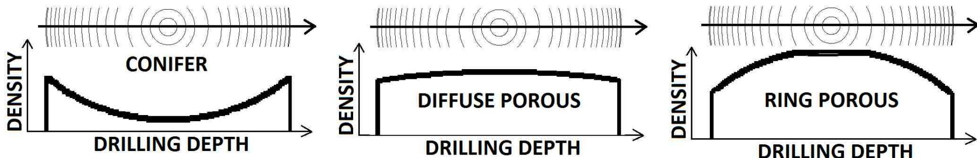
(can be measured and correctly displayed by x-ray densitometry or, for example, by resistance drills, but only by calibrateable machines -versions)
