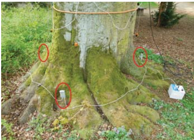
Figure 7. Three sensors were placed at the base of a beech tree ( Fagus sylvatica ). One in the pulling direction, one opposite and one at a 90° angle. The resulting tilting curves differed significantly and would have led to three correspondingly different final estimations of uprooting safety.
