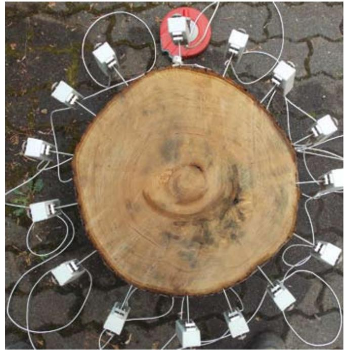
Figure 4. (Right) For scientific purposes, 15 stress wave sensors were placed around the stem for obtaining a sonic tomogram picture. In a 'real' world inspection, for such a cross section, typically 8 to 10 sensors would be used and sufficient.
