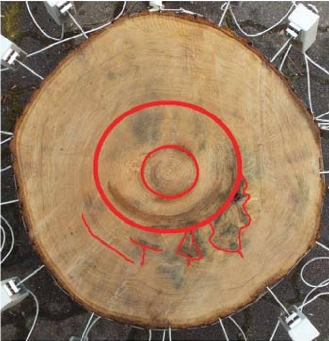
Figure 3. (Left) The red circles indicate the decayed tree-rings (ring-shake). In addition, some small areas showed remains of previous damages (marked red).
