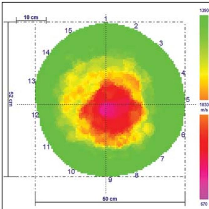
**Figure 6.** Based on the line graph, a special computer program automatically calculates a 2d-tomogram picture visualizing the internal situation: this does not and cannot, in general, reveal overall local wood condition but just shows the remaining (wind-) load carrying parts in green (these are the intact and mechanically interconnected parts of the cross section).
