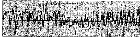
Figure 11 RESISTOGRAPH-profile of Fagus sylvatica (feed rate = 280 mm/min, right to left, vertical dotted lines = 10 mm steps). Narrow rings dominated by earlywood lead to decreasing profile level, revealing the radial density trend.
