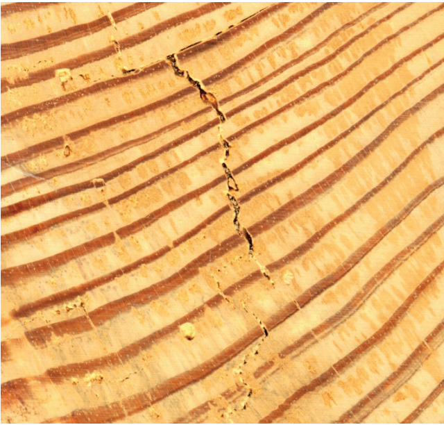
Fig. 2: This more detailed close-up of Fig. 1 shows the spotted areas of early brown rot decay of the broken Pinus ceiling beam. In this stage, obviously only early-wood is affected as can be seen by the location and size of the decayed areas. Resistance drills thus have to provide high resolution and linearly scaled, calibratable profiles in order to enable the experienced user to identify such decay in the curves. As in this example, although the decay is in an early stage, the consequences of bending strength loss can be severe.
